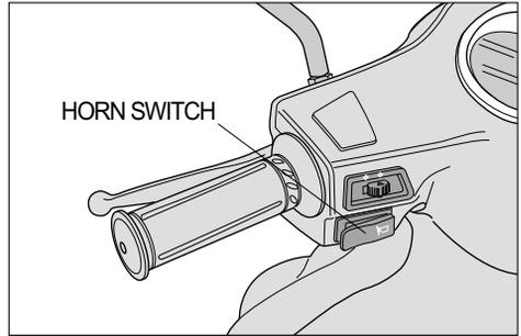
Press the switch to operate the horn.
