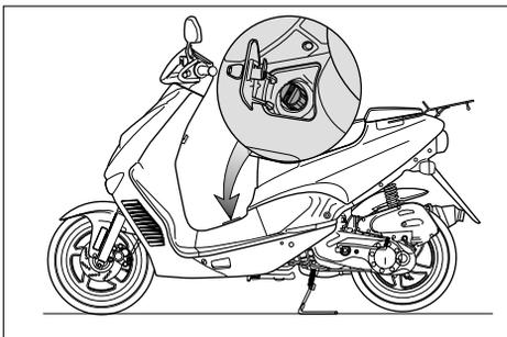
1. Insert the ignition key into the lock located a center of the footboard and turn it counterclockwise.
