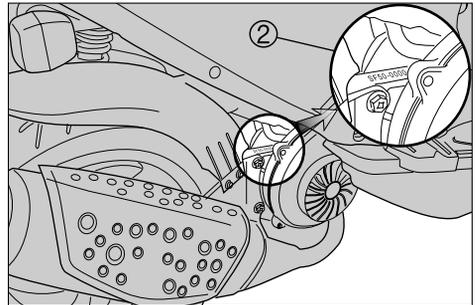
The frame number ① is stamped on the right side of the frame under the footboard.
