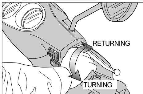
You can adjust the speeds with the throttle grip.
