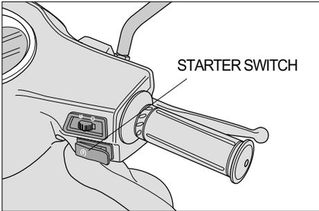
Push in the electric starter switch to rotate the starting motor.
