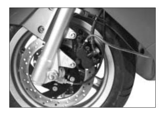
Squeeze and release the brake lever several times in rapid succession and sqeeze the lever fully without releasing it. Loosen the bleeder valve by turning it a quarter of a turn so that the brake fluid runs into the receptacle, this will remove the tension of the brake lever causing it to touch the handlebar grip. Then, close the air bleeder valve, pump and squeeze the brake lever, and open the valve. Repeat this process until the fluid flowing into the receptacle no longer contains air bubbles.
