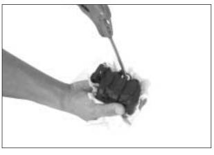
• Remove the dust seal ① and piston seal ②.
