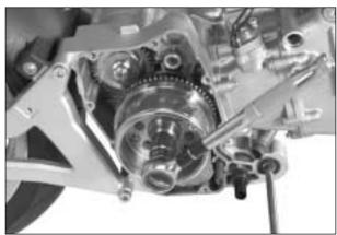
• Remove the magneto rotor② by using the special tool.
